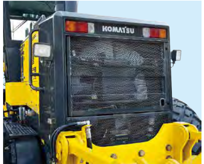
Hydraulic driven cooling fan
