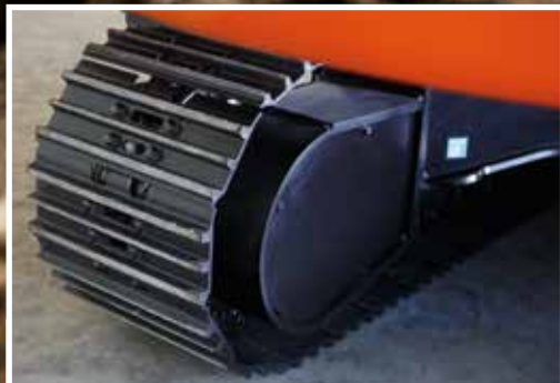
Risk of damage is reduced by a reinforced motor cover.
